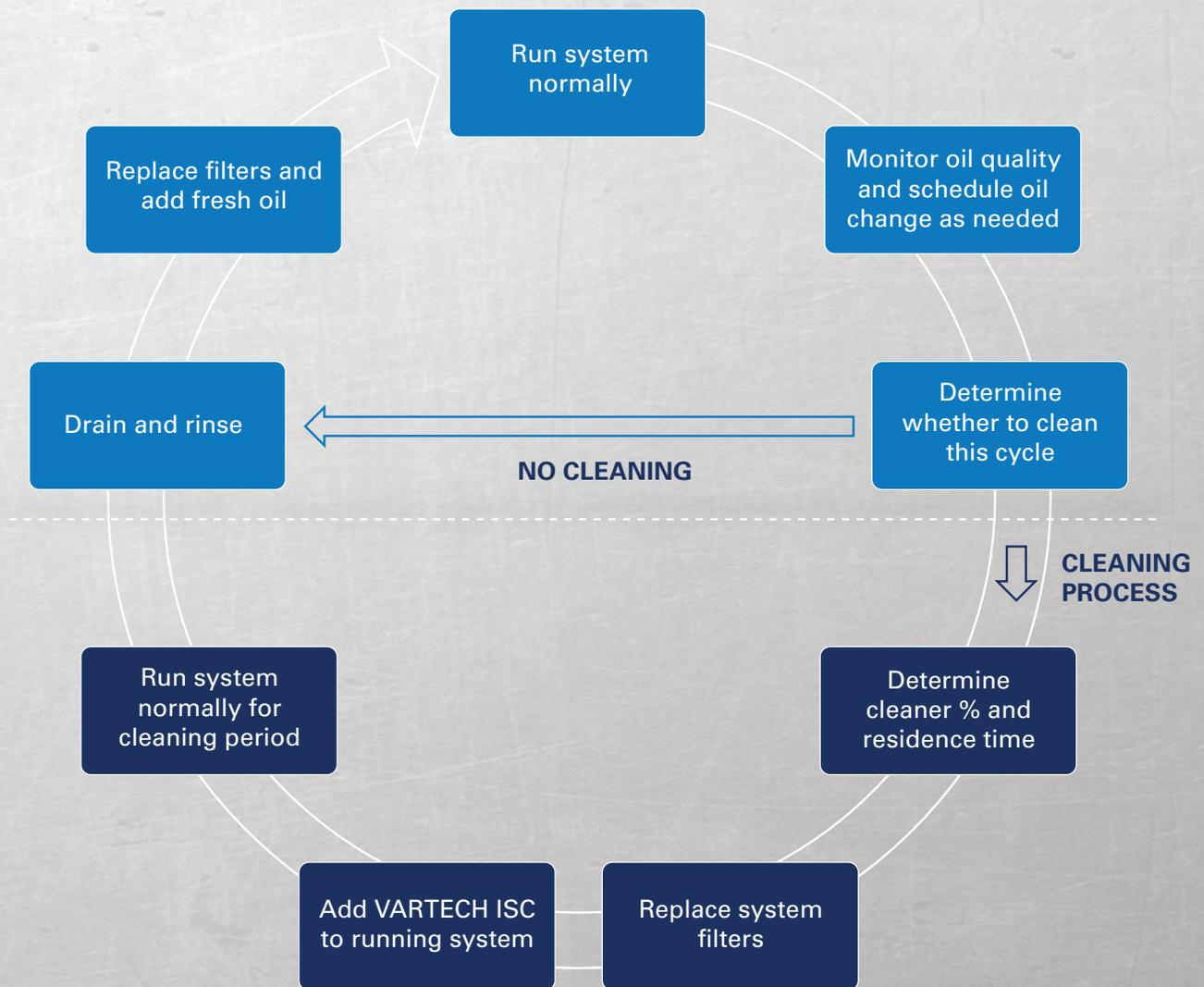
The VARTECH™ Industrial System Cleaner (ISC) cleaning process is simple, streamlined and economic. Conventional system cleaners are more complex and require additional steps, external filtration and multiple rinses and compatibility tests.
